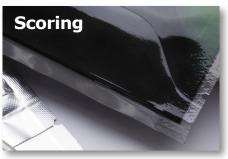
200 Watts average laser power delivers precise scoring at high speed, perfect for flexible packaging production lines. Digital control enables on-the-fly changes, reducing production downtimes associated with traditional die pattern change-overs.
