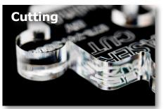
The f201 excels at acrylic cutting, delivering smooth, polished edges in a single pass. Digital control, exceptional power and divergence stability enable detailed cuts, with change-on-the-fly capability.
